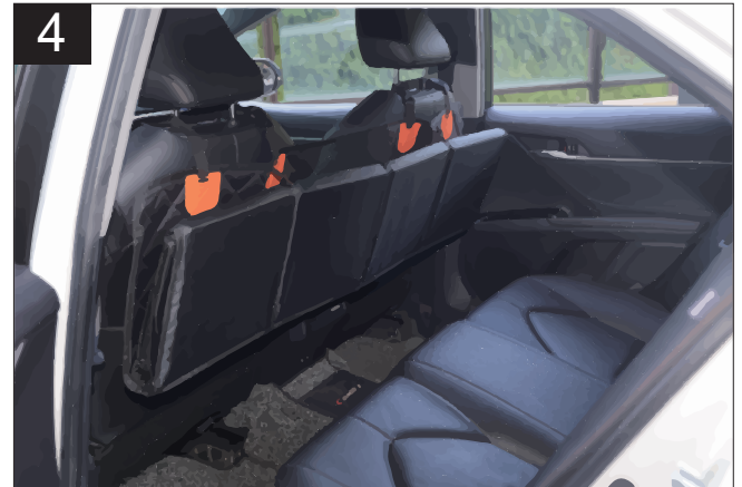
Step 4- Attach the loop strap on the back of the seat cover to the button on the front seatback.
